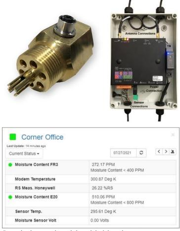
Example alarm on the web-based dash board.
